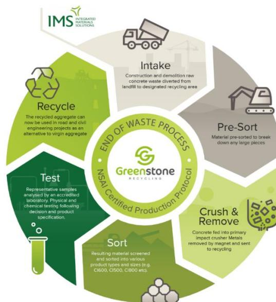
Fig 2: Process of turning waste concrete to a useable aggregate
